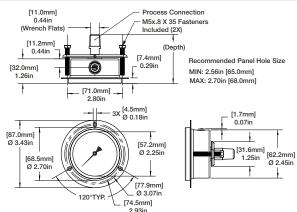
63 mm center back connect - front flange, case mounted U-clamp **Connection Code Process Connection** Depth 01 1/8 NPT 2.36 [60.0] 02 1/4 NPT 2.50 [63.4] 13 G¼ B 2.49 [63.3] 41 M14x1.5 2.53 [64.3] EJ JIC #4 2.44 [62.0] JP 1/4 Tube 2.60 [66.1] JR 3% Tube 2.73 [69.4] JS 1/2 Tube 2.86 [72.7] 1/4 BSPT KA 2.42 [61.4] SAE 7/16-20 RW 2.60 [66.1] [49.2mm] Process Connection
