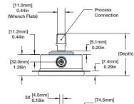
Recommended Panel Hole Size MIN: 2.56in [65.0mm] MAX: 2.70in [68.0mm]
