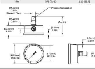
63 mm center back connect - connection mounted U-clamp **Connection Code Process Connection** Depth 01 1/8 NPT 2.36 [60.0] 02 1/4 NPT 2.50 [63.4] 13 G¼ B 2.49 [63.3] 41 M14x1.5 2.53 [64.3] JIC #4 EJ 2.44 [62.0] JP 1/4 Tube 2.60 [66.1] JR 3% Tube 2.73 [69.4] JS 1/2 Tube 2.86 [72.7] KA 1/4 BSPT 2.42 [61.4] RW SAE 7/16-20 2.60 [66.1]
